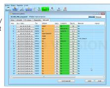
The security system stores all performed operations and events (setting, unsetting, alarms, faults, messages sent to users and ARCs) in the micro SD card in the system's control panel. Each entry includes the date, time (start and end), and source (cause / origin) of the event.
