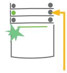
2. Press the right button (the one which isn't lit up) to set a particular section. It is possible to set more sections subsequently. The delay between sections selection must not be longer than 2 seconds.
