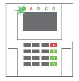
3. The command is executed and the keypad acoustically indicates the exit delay. The section is set now, only the detectors with a "Delayed Zone" reaction provide time to leave the guarded area during the Exit delay. The status indicator and a function button of the set section will turn red.
